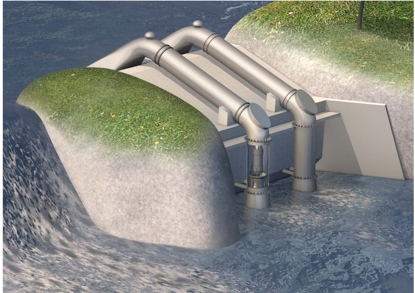
Penstock Siphon Example
